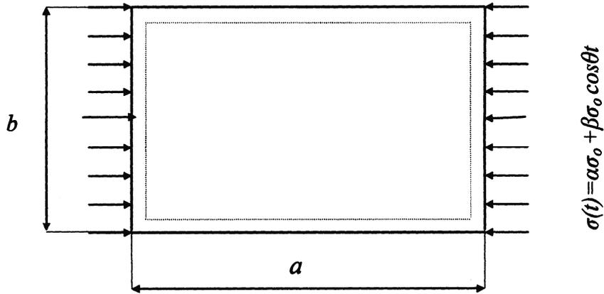
Fig. 1. Plate supported in a jointed way on the circumference
