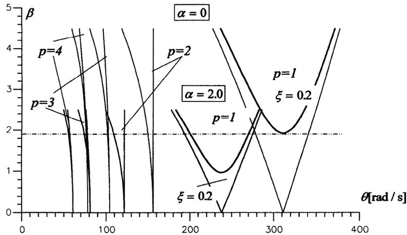
Fig. 3. Limits of regions for  $p=1, 2, 3, 4$  of the first resonance frequency at initial load  $\alpha = 2.0$
