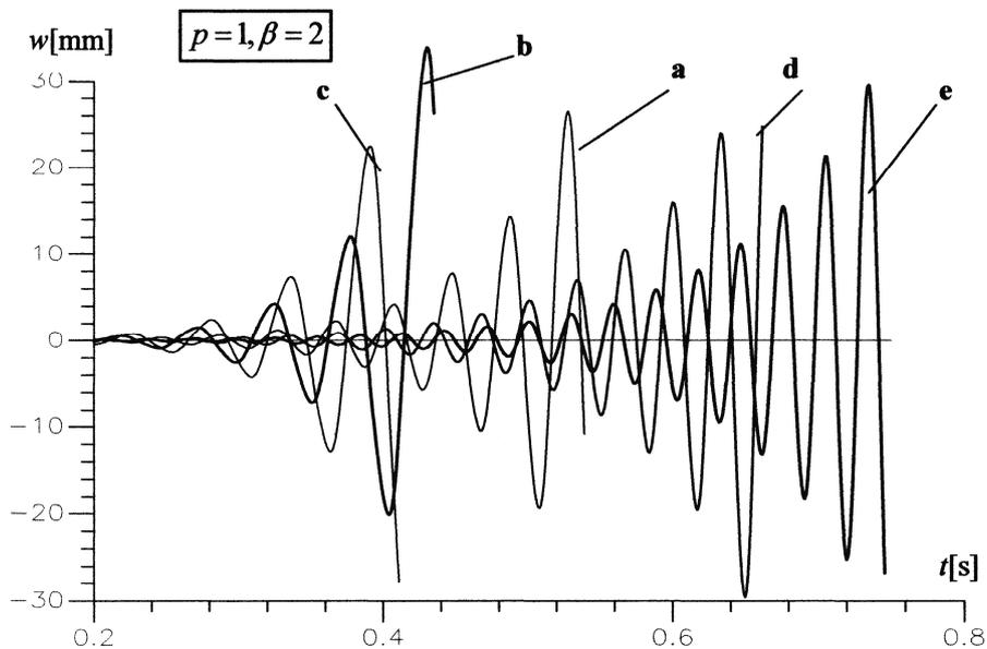
Fig. 5. Plate vibration diagrams at different initial load
